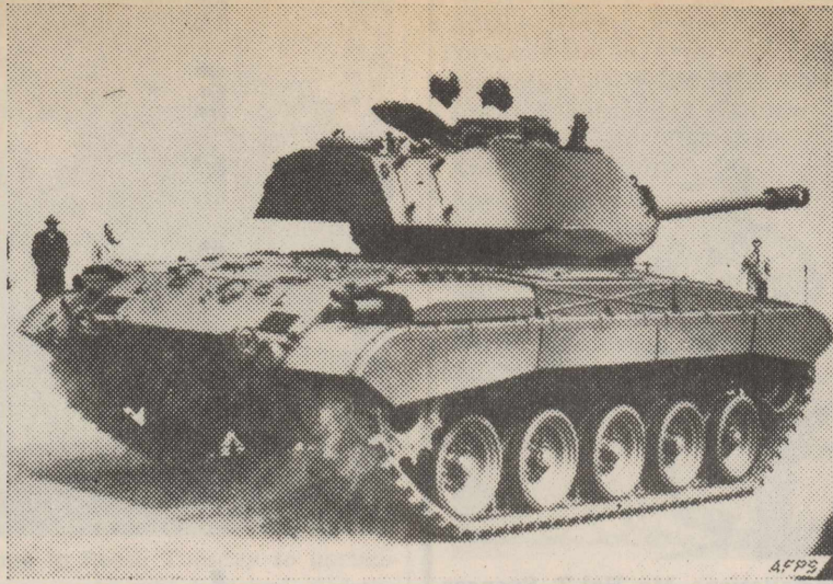
THE LIGHT T-41, or Walker Bulldog, first tank produced by a civilian company since World War II, has begun rolling off the assembly lines at the Cleveland Airport Bomber Plant, three months ahead of schedule. Named for the late Gen. Walton H. Walker, 8th Army Commander, the 26-ton tank sports a new type high muzzle velocity 76 mm. gun.
