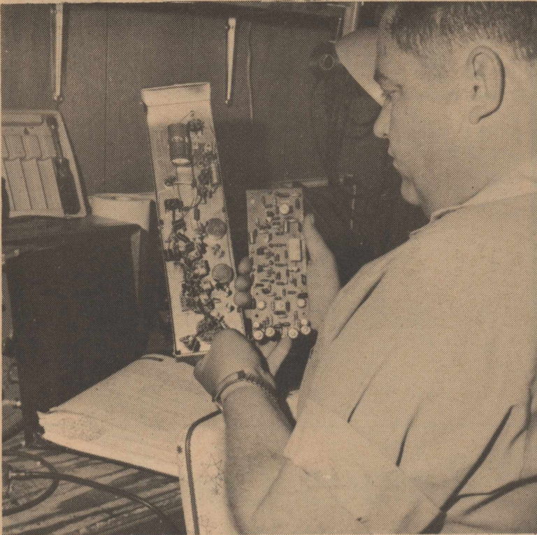
Lloyd Coberly, engineer for TV Cable of Seminole, is shown in the above picture with a line extender in his right hand and a trunk line amplifier in his left hand. Mr. Coberly was discussing the TV cable service and pointing out some of the problems they'd had. "I do hope," he said, "we will have the tower completed in February." As an example of the things that can go wrong with the cable system they have installed sixty-five line extenders. A line extender measures 3"x8", has 111 parts and costs $360.00. If any one of the 111 parts go out someone has trouble. Besides the line extenders that have been installed fourteen trunk line amplifiers have been put in at a cost of $450.00 each and sixteen bridge amplifiers. "We hope to finish the new construction at a cost of about $100,000.00." When the rework is finalized Channel 2 will be 2 on the selector, Channel 7 will be 7, Channel 10 will be 10 and also others will change.
