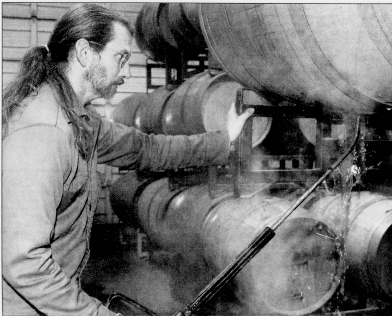
Morrell Taylor, a Llano Estacado Winery employee, cleans solid deposits from wine barrels using hot water.
