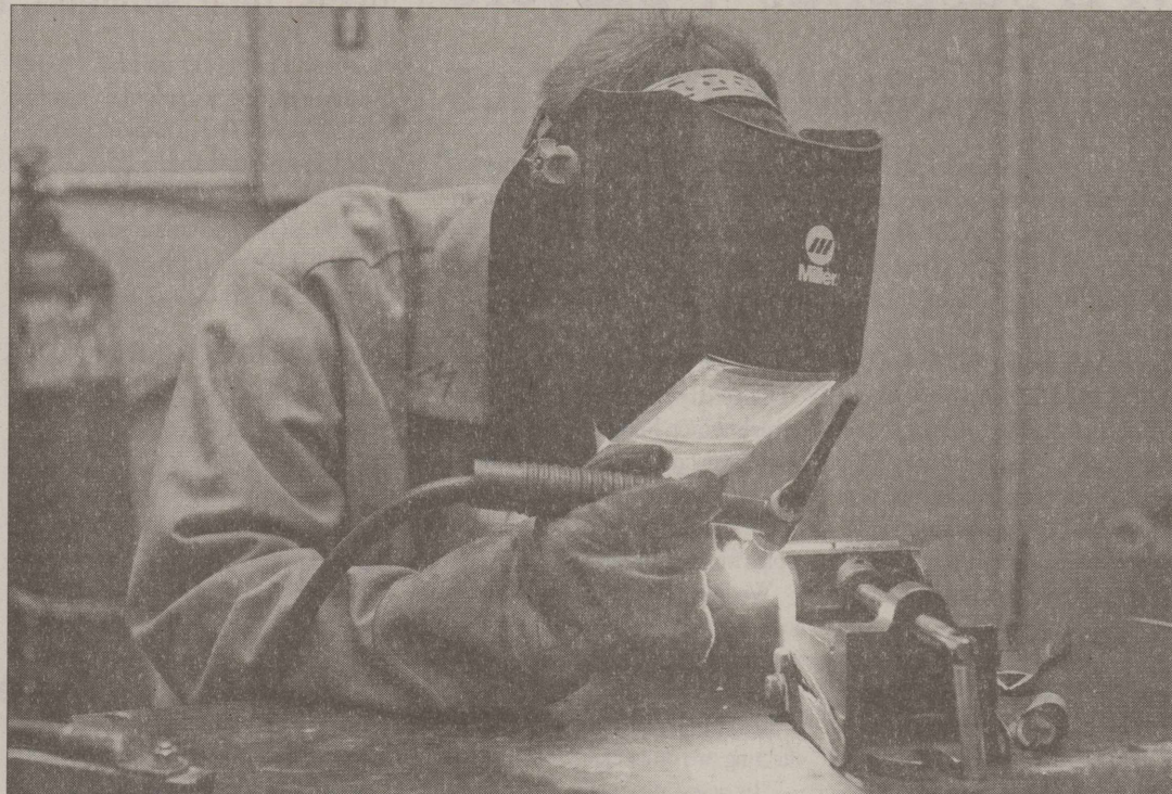
PHOTO BY SCOTT MACWATTERS/The Daily Toreador JEFF BOUVIER, A sophomore mechanical engineering major from Austin, welds together a radiator hose in the Mechanical Engineering building Wednesday. The radiator hose will be used in a formula car for a competition hosted by the Formula Society of Automotive Engineers next week in Brooklyn, Mich.
