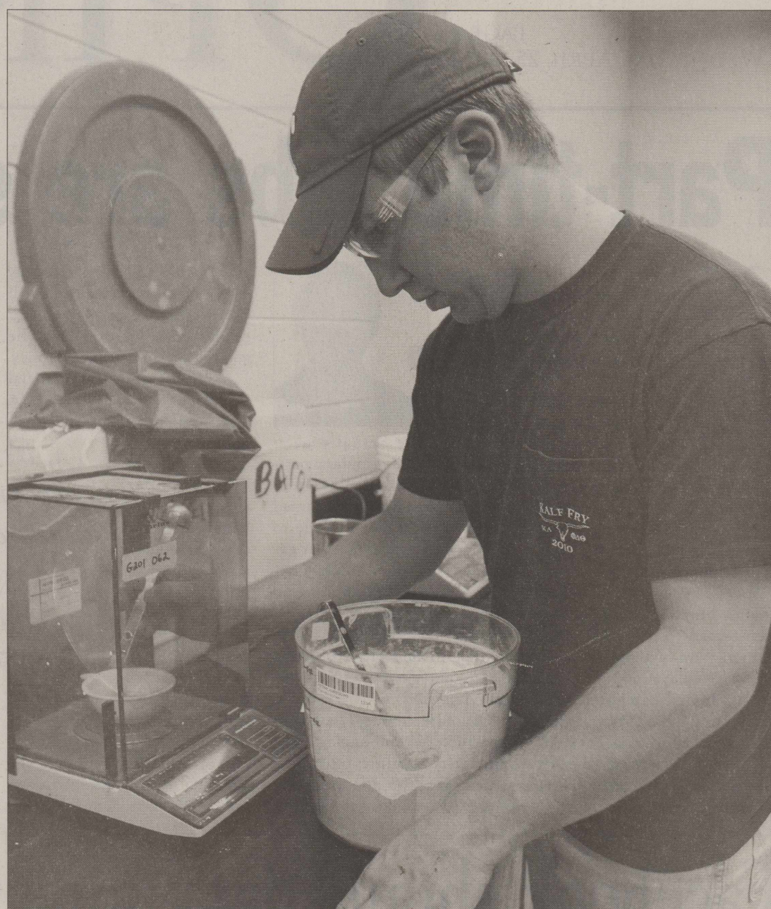
PHILLIP RANDEL, A junior petroleum engineering major from Nacogdoches, weighs out bentonite for a drilling sample during a mud lab Monday in the Petroleum Engineering building.
