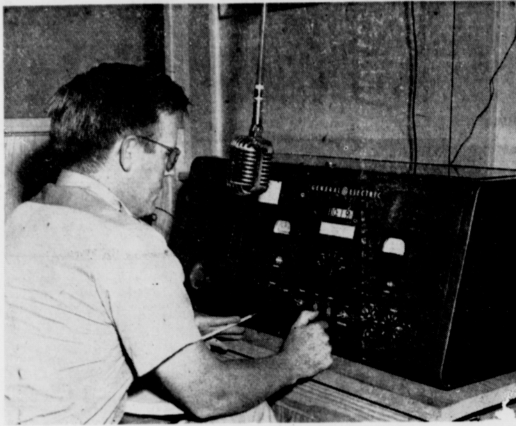
Billy Woods, dispatcher in the Abilene electric distribution office, operates WTUCo's new central 250 watt, FM radio station, KHIQ. Above Woods is pictured taking an incoming call from a line service truck over the two-way radio system. The WTUCo. now has seven vehicles operating out of Abilene and Cisco which are equipped with mobile 60-watt two-way radios.
