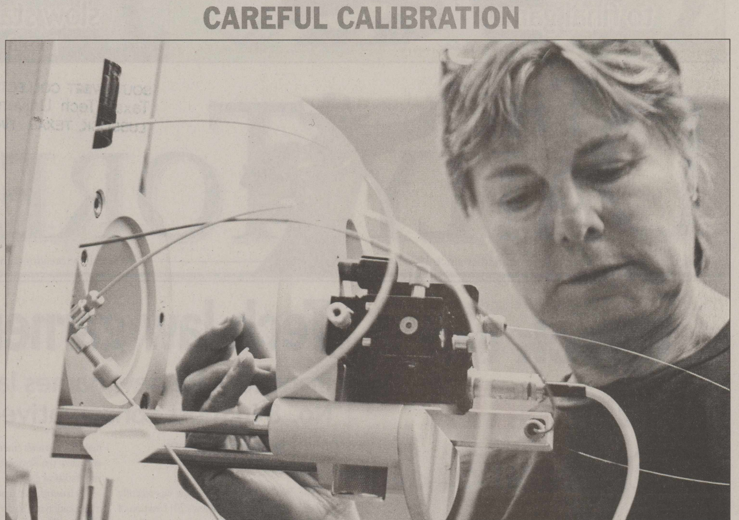
SUSAN SAN FRANCISCO, a research associate for the center for biotechnology from Lubbock, measures the flowrate of a nano column to calibrate a mass spectrometer in the Experimental Sciences building on Monday.
