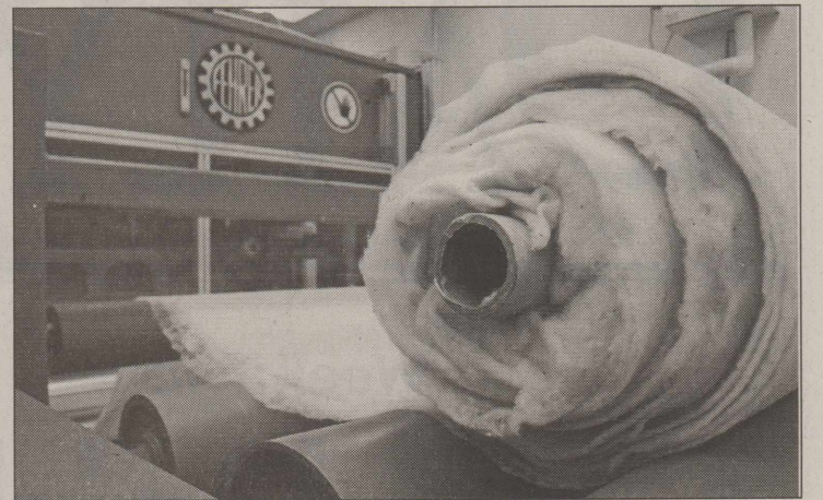
PHOTO BY BRAD TOLLEFSON/The Daily Toreador A FINISHED ROLL of nonwoven cotton gathers at the output of the needle punching line at the Nonwovens and Advanced Materials Laboratory at the Institute of Environmental and Human Health.
