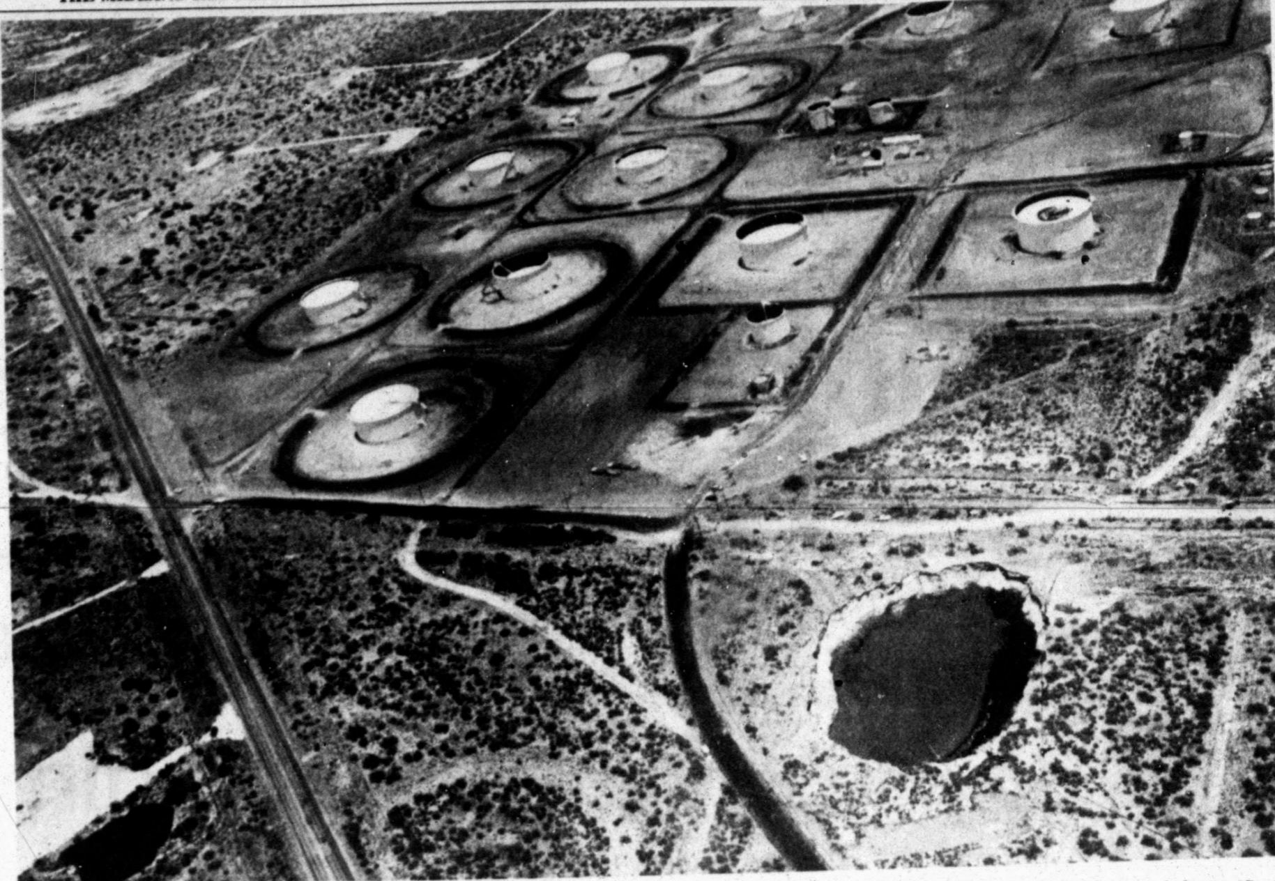
Measurements show the Kermit "crater," bottom right, to be slowing in its growth toward a Shell Oil Co. tank farm and State Hwy. 115, shown running diagonally at the far left.
