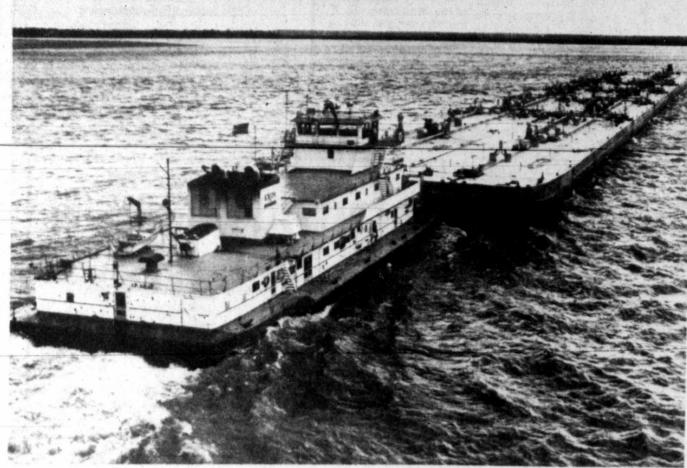
Moving 185,000 barrels of petroleum products on the Mississippi River 15 miles south of Memphis, Tenn., this Exxon Co., U.S.A. river boat is six times more fuel-efficient than the 480 trucks it would take
