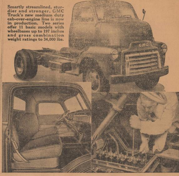
LEFT: The new C.O.E. cab features all of the comfort and convenience advancements found in GMC's 1948 conventional models. All-steel and 61/2 times stronger than prewar, it provides a revolutionary ventilation system, 22 per cent more vision, 8 inches more seating width with nearly twice the number of seat springs and complete insulation.
