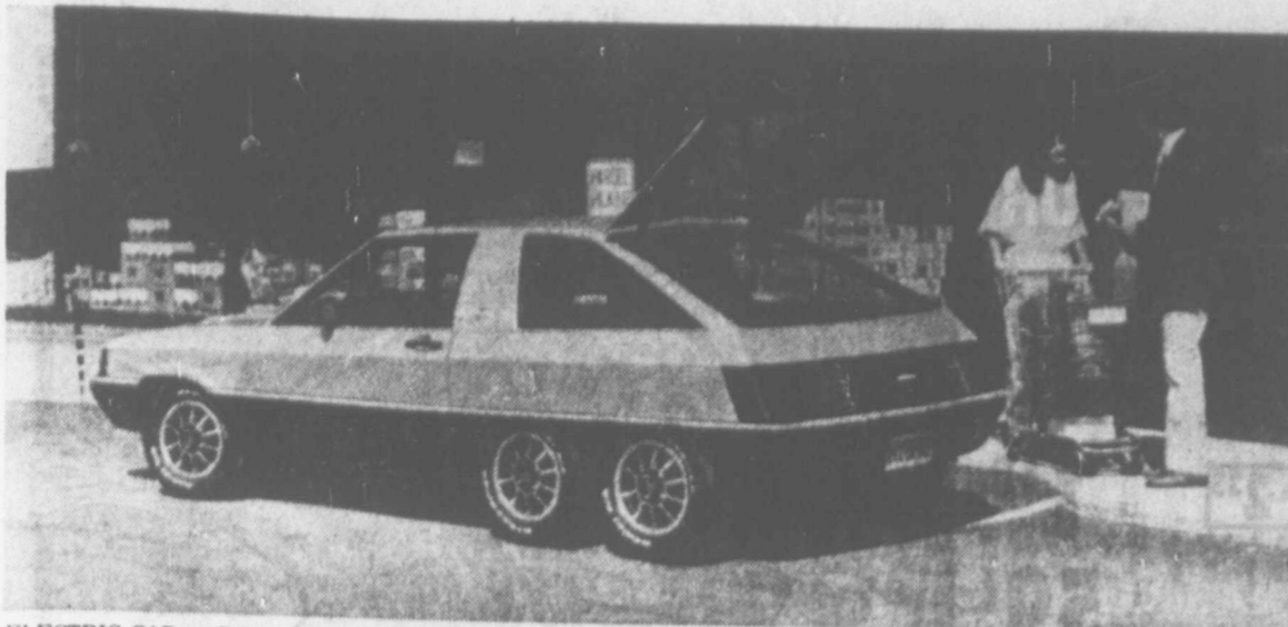
ELECTRIC CAR — Briggs & Stratton, builder of small gasoline engines, has unveiled this six-wheeled that can be propelled by its electric motor, an 18-horsepower gasoline engine, or both powerplants in unison. The firm says gas mileage varies between 25 and 150 miles per gallon. The car was designed to carry two adults, two children and two bags of groceries. (AP Laserphoto)
