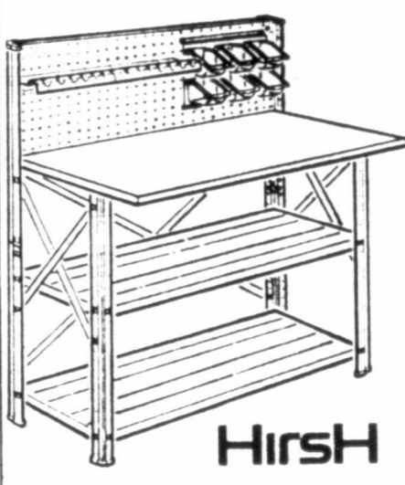
Hobby Bench 20x36" work surface with 2 bottom shelves, tool rack, perforated backboard and 6 removable bins. #TW108
