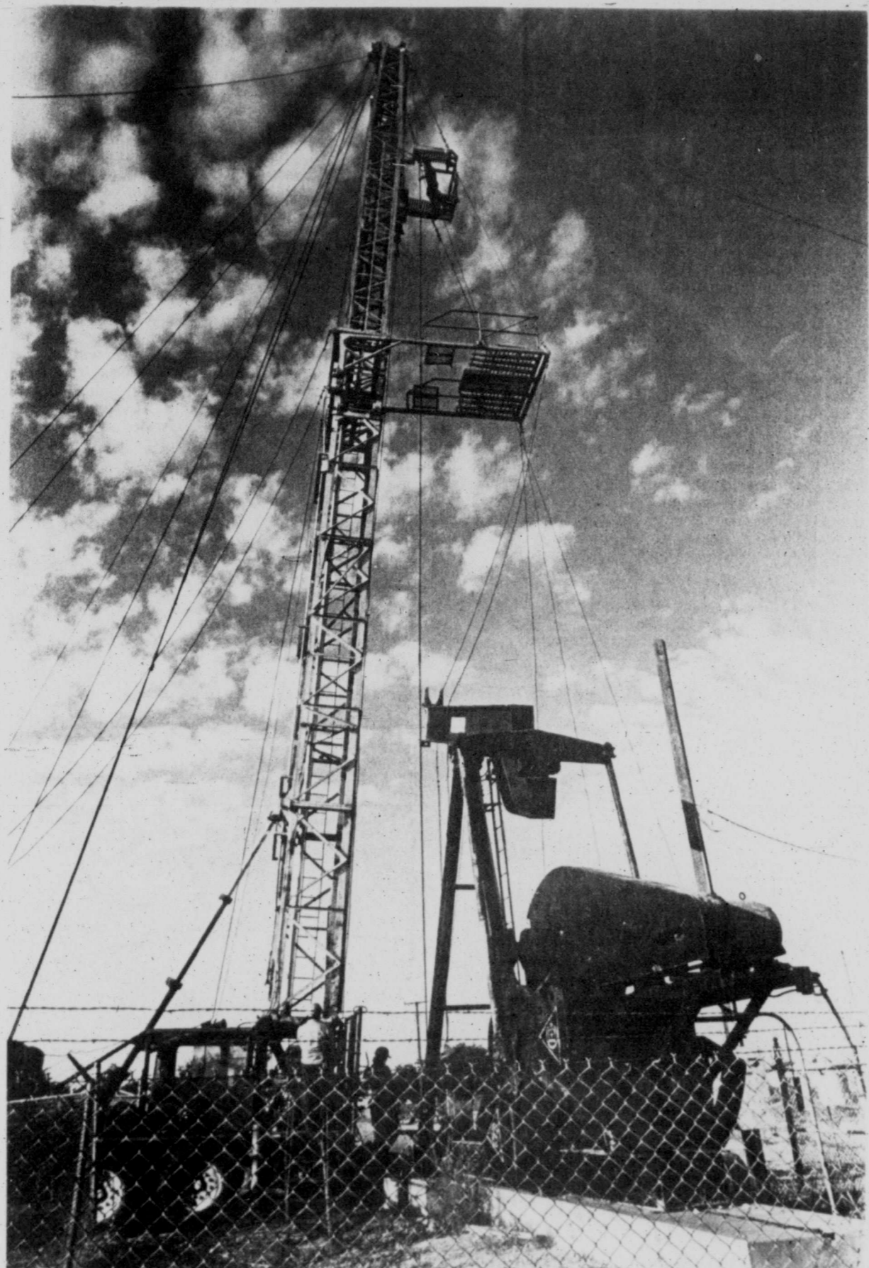
Workers replace pumpjack rods at the No. 1 Inez Faskin oil well owned and operated by Miller Exploration Company of Midland. Located in the 100 block of South Eisenhower Drive, the well reportedly is the only producing one within the Midland
