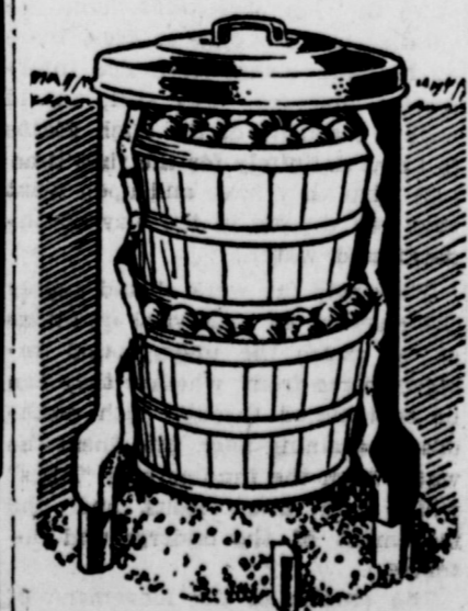
Drawing shows method of installing section of vitrified clay pipe for use as storage pit for fruit, eggs, milk and vegetables. Note that bell rests on bricks. Spigot end should protrude above ground two inches so dirt fill will slope away from opening. At bottom is layer of coarse drainage material. Top opening covered with gravel screen or with wood or metal lid.
