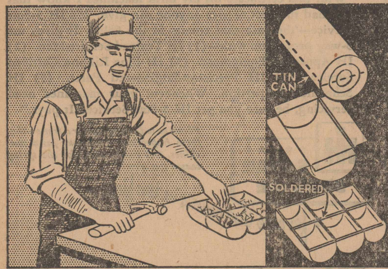
SECTIONAL TRAY . . . Discarded tin cans of uniform size, preferably the type in which condensed milk is sold, can be cut in the manner indicated in drawing and then crimped and soldered together to make storage trays that will be useful for storing various small parts.
