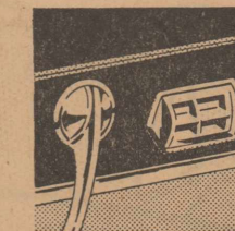
New Electric Window Lifts raise or lower front windows to any desired height by simply touching a button.
