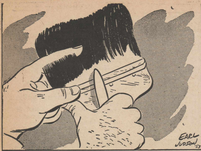
TRIM OLD BRUSHES . . . Worn bristles on the outer row of a paint brush destroy the brush's flexibility. Use a sharp knife or razor to trim away this outer row and give the brush new life.
