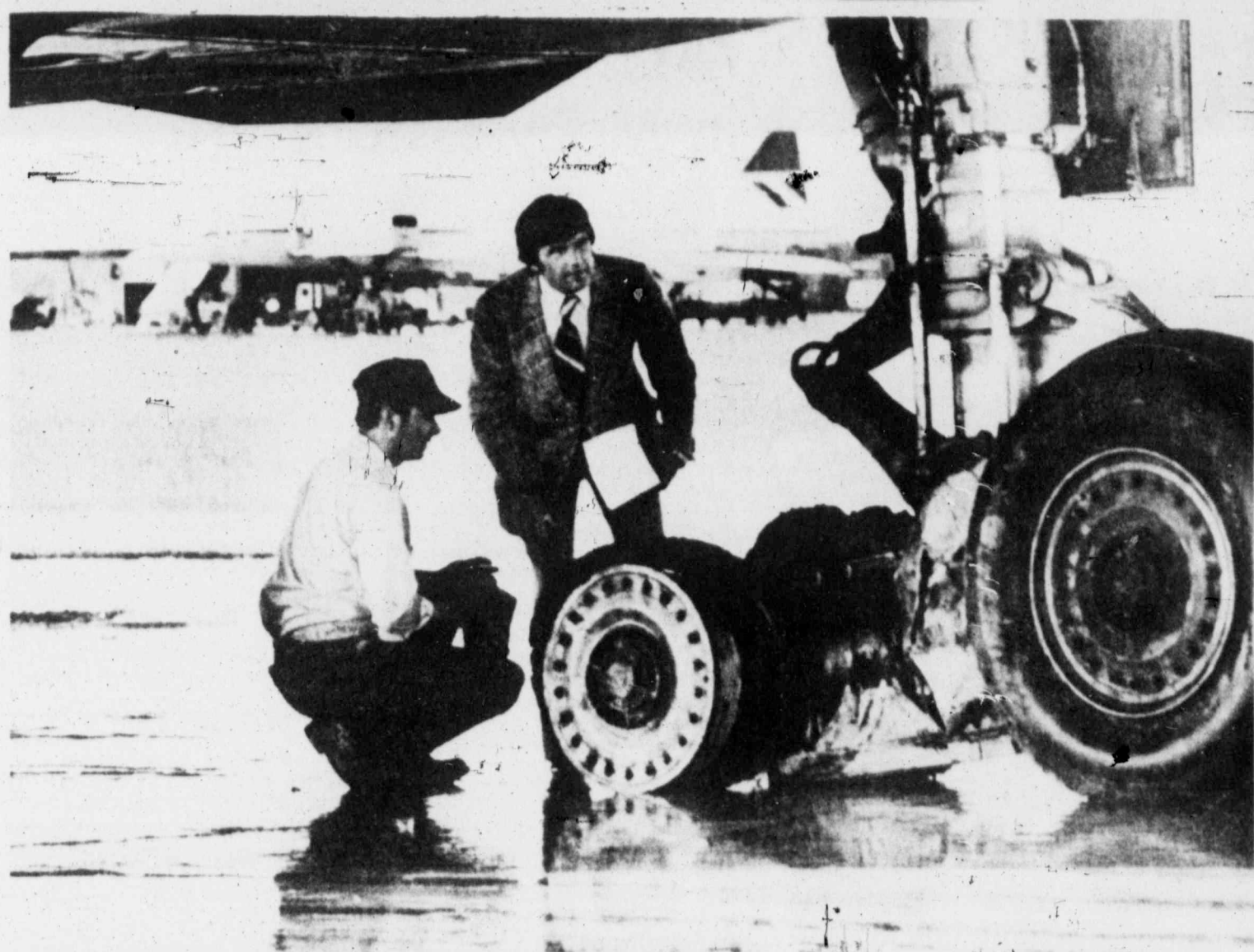
Technicians inspect damage on an Air France supersonic Concorde which blew two tires and ruptured a fuel tank on take-off from Dulles International Airport outside Wash-
