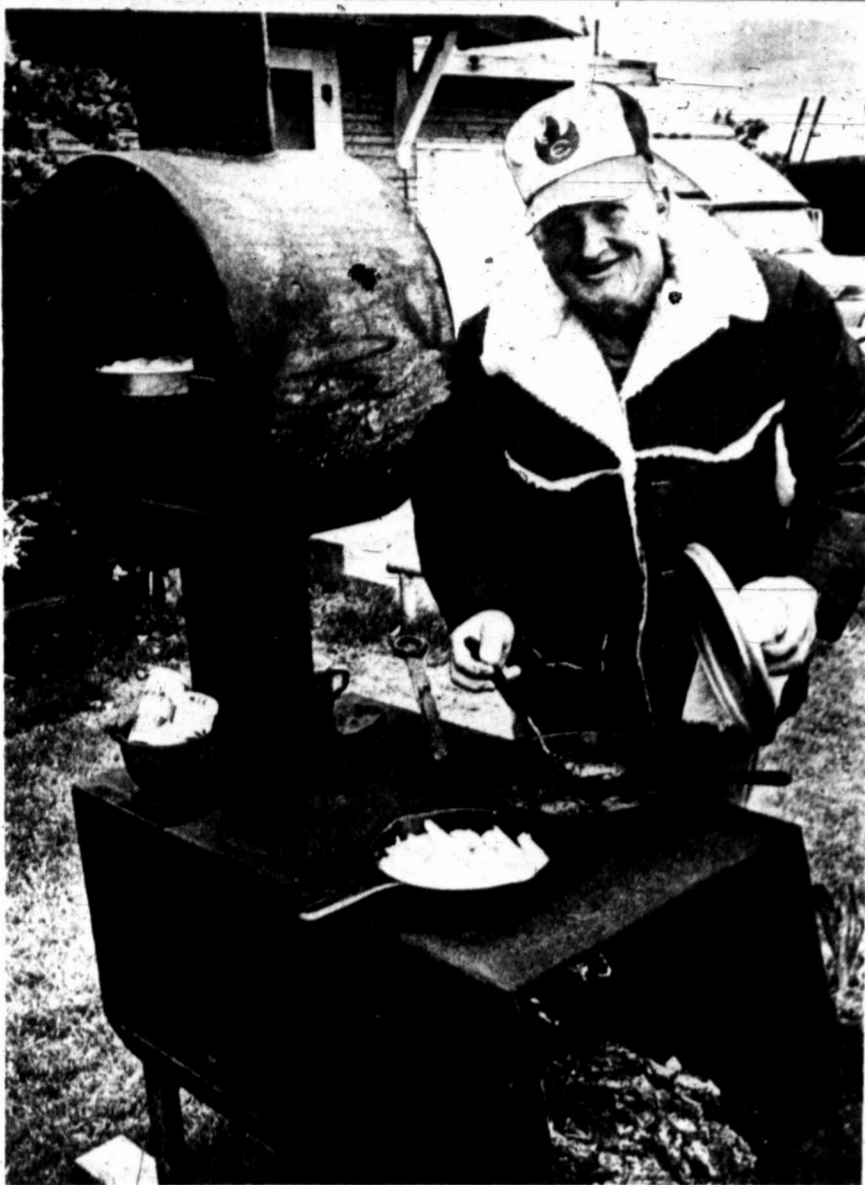
Cooking some meat, potatoes and biscuits on an old fashioned wood-burning stove and oven he designed and built is Midlander Onis E. Kelton. A welder by trade, Kelton fashioned his creation from 3/8-inch thick steel pipe and plate. He claims it should last a lifetime. (Staff Photo by Brian Hendershot)
