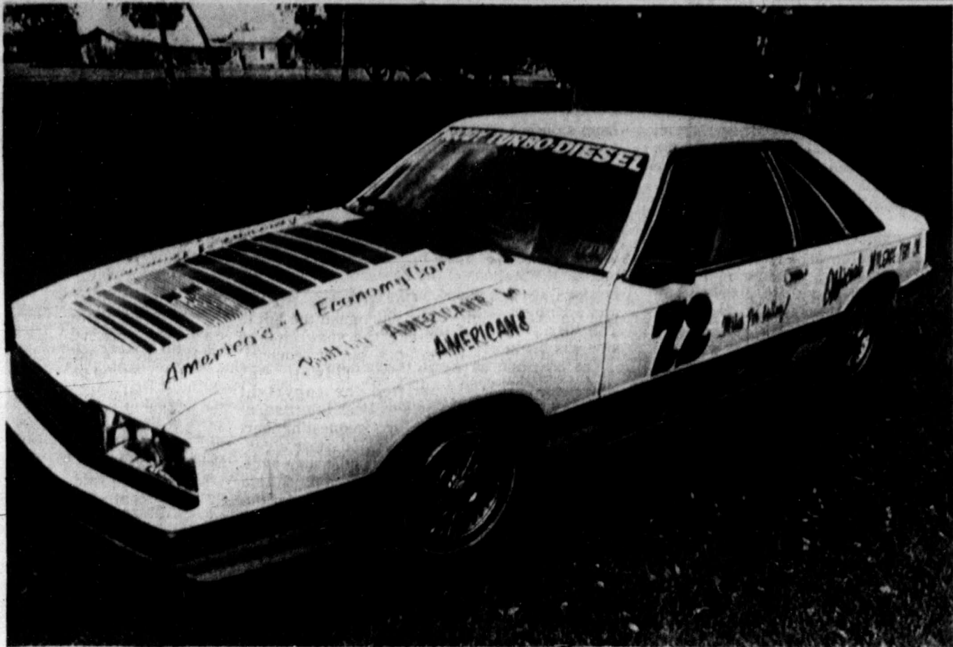
Ralph Moody, former Ford Motor Co. racing division head, and Mike Shetley have redesigned this 1979 Mercury Capri, enabling it to travel over 80 miles on a gallon of gasoline. Their original
