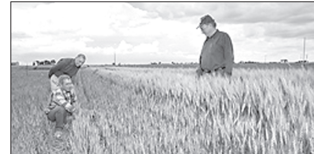
ARS agricultural engineers Walter Bausch (foreground), Gerald Buchleiter (right), and Laj Ahuja evaluate the distinct differences in wheat growth at full irrigation (right side) and 40 percent of full irrigation.
