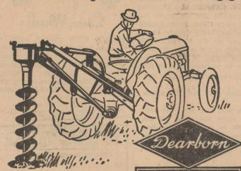
Why wait to build fence because digging post holes by hand is such hard work? We recommend the Danuser post hole digger that attaches quickly to the Ford Tractor and can dig up to 600 post holes a day. Lifts and lowers by Hydraulic Touch Control. Pays for itself in time and labor saved . . . gets fence made quickly, between rush seasons or in spare time.
