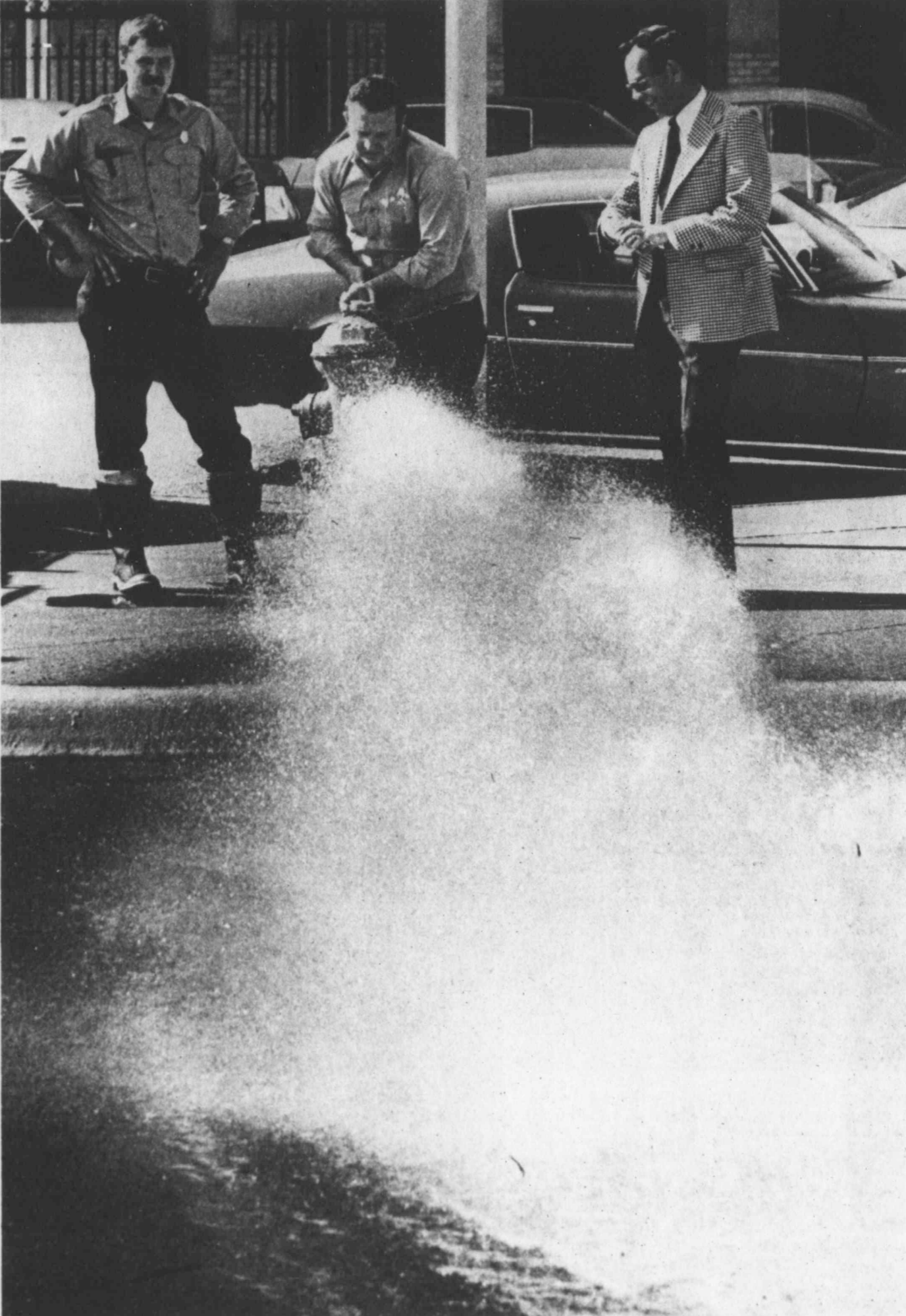
Firemen, from left, Gary Glass and S.L. Vann assist Dallas insurance consultant Floyd E. Creasey Monday as he tests pressure and resistance of water spouting from a hydrant at the corner of Illinois Avenue and Baird Street. Creasey's firm was in Midland testing several hydrants "so we'll be sure there's enough water to keep our clients' (structures) from burning down."
