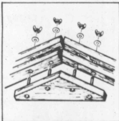
Rigid Frame Construction
