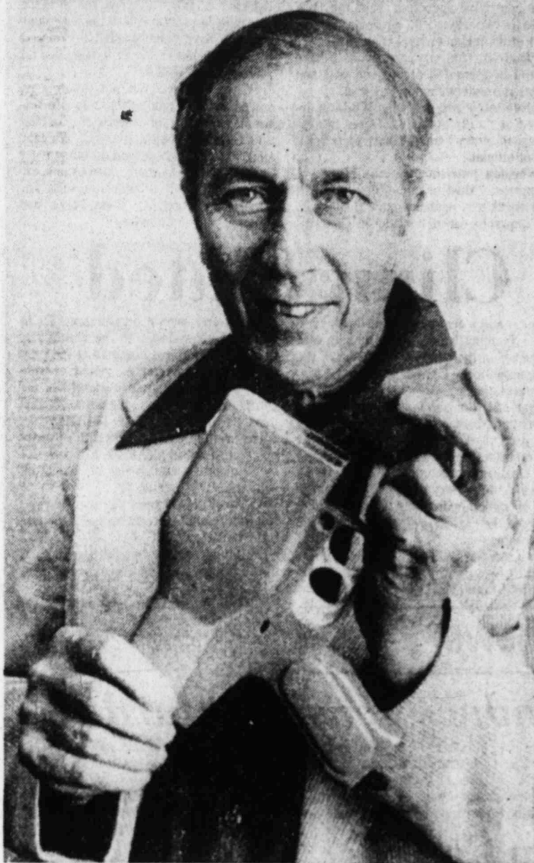
DEFENSE WEAPON — Frank Cover, president of Taser Systems, Inc., of the City of Industry, Calif., holds a taser, a type of defensive weapon, in one hand and its cartridge in the other. The taser, utilizing an electrical charge, generates an electrical current that induces involuntary muscle contractions. (AP Laserphoto)
