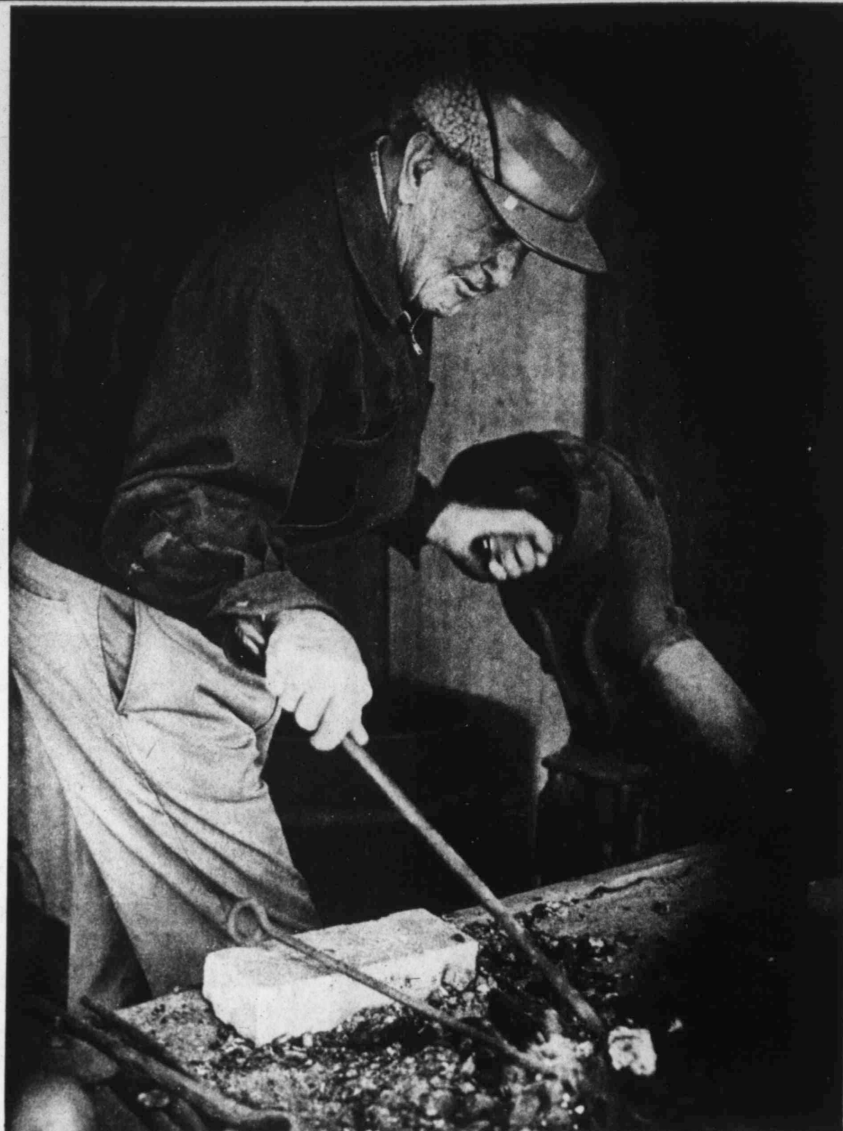
Working an air pump with his left hand to keep the coals red hot, the blacksmith nudges still-solid aluminum into a bull plug he uses as a crucible.
