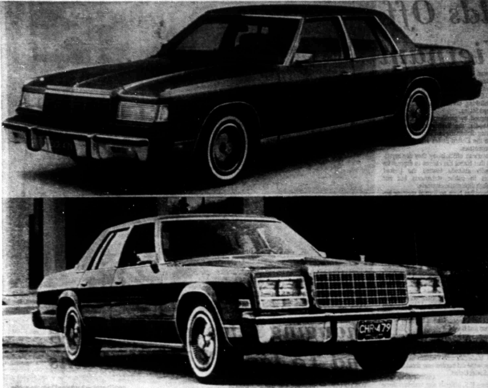
CHRYSLER'S FULL-SIZE LINE — Here are two of the three full-size cars offered by Chrysler Corp. for 1979. Top, The Dodge St. Regis and, bottom, the Chrysler Newport. Both cars are about seven inches shorter, two inches narrower and 700 pounds lighter than 1978 versions. The Newport and St. Regis will have a two-barrel 225-cubic-inch six-cylinder engine standard. (AP Laserphoto)
