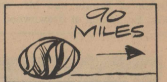
A fiber 90 miles long can be drawn from one glass marble less than an inch in diameter.
