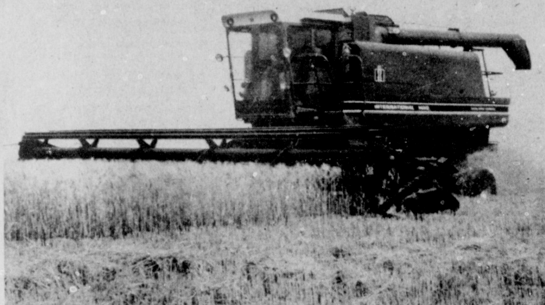
INTERNATIONAL HARVESTER'S AXIAL-FLOW COMBINE—International Harvester's Axial-Flow combine harvested more wheat per unit area at both high and moderate feed rates during comparative tests with conventional machines. At moderate feed rates on four series of trials, conducted by Kansas State University agricultural engineers, the Axial-Flow averaged a 4.5% yield advantage. The IH machine also consistently caused less crackage in all varieties of wheat harvested, the engineers reported.
