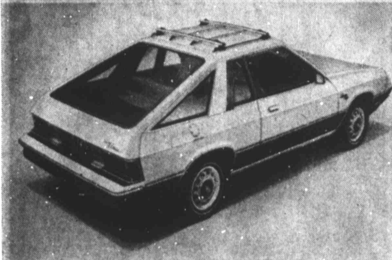
NEW ADDITION TO HORIZON LINE — The newest addition in the Plymouth Horizon line for 1979 is a sporty hatchback, the Horizon TC3. Like the standard four-door model, it has front-wheel drive and transverse-mounted four-cylinder engine. The aerodynamically styled TC3 hatchback is about eight inches longer and nearly 2 1/2 inches lower than the four-door Horizon. (AP Laserphoto)
