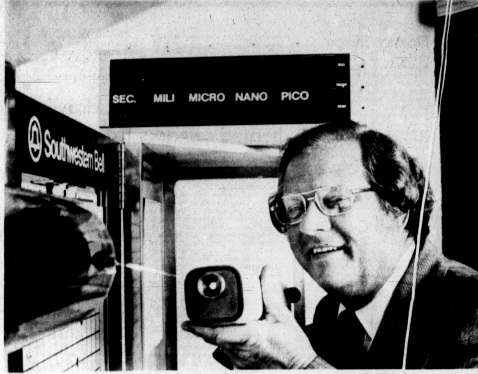
FASTER than a speeding bullet, Bill Haehnel explains, lasers are used to transmit telephone calls along glass light fiber. The light fiber, which is hair-thin, is less bulky than the copper cables now being used by Southwestern
