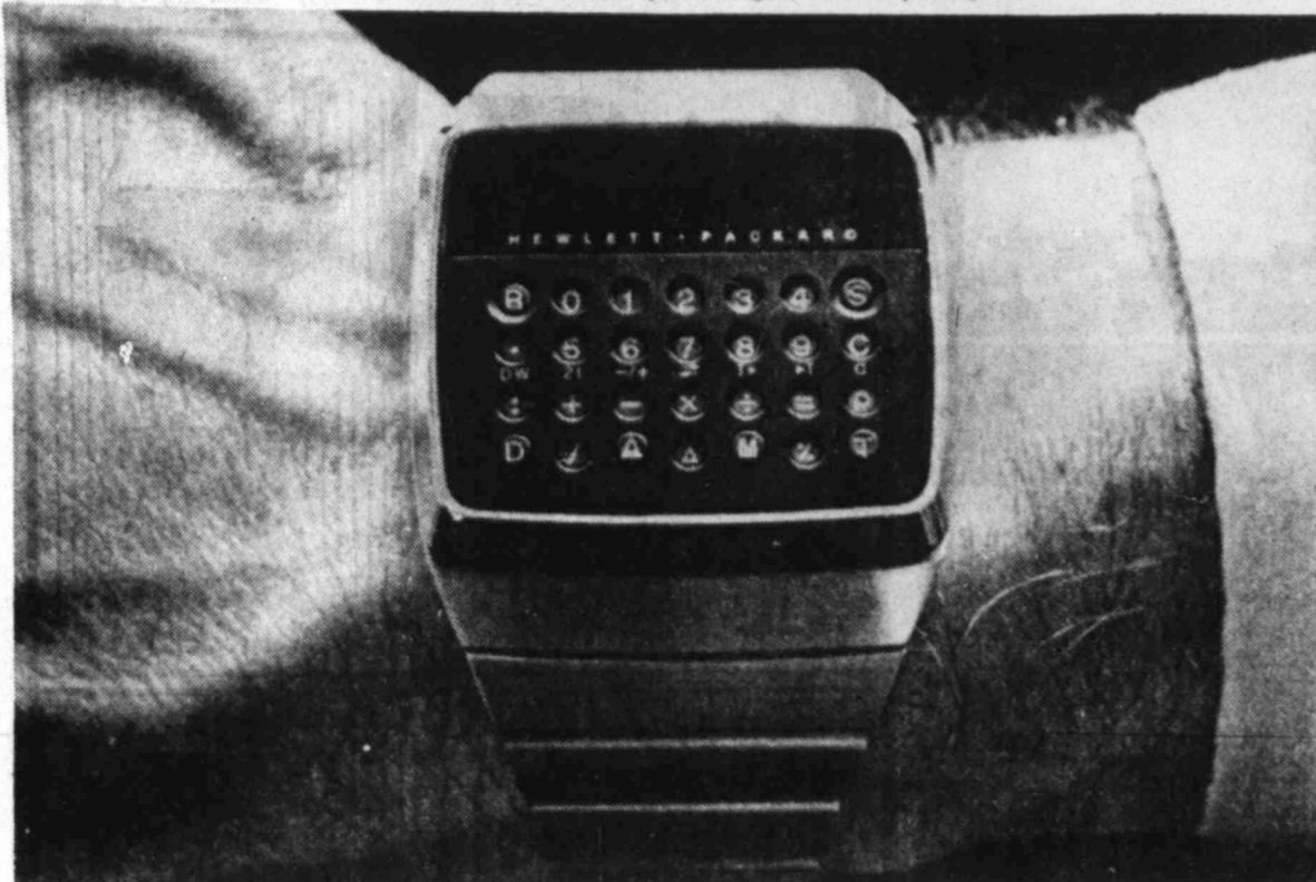
SPACE AGE WATCH — This is the Hewlett-Packard HP-01 as part of the dazzling package. (AP Laserphoto) that not only tells time but offers a 200-year perpetual calendar
