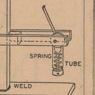
Because of its quick action, the Australian clamp has several advantages over the screw type. One advantage is that the job does not move when the clamp is put into action; another is that it eliminates worry about splashing metal on threads.
