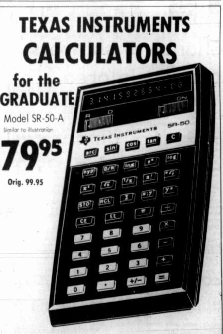
SLIDE RULE CALCULATOR ... The Texas Instruments SR-50A slide-rule calculator performs roots, powers, reciprocals, factorials, common and natural logarithms and inverses, trigonometric and hyperbolic. functions and inverses, all in floating decimal or Scientific Notation. Easy to use single-function keys plus memory capability:
