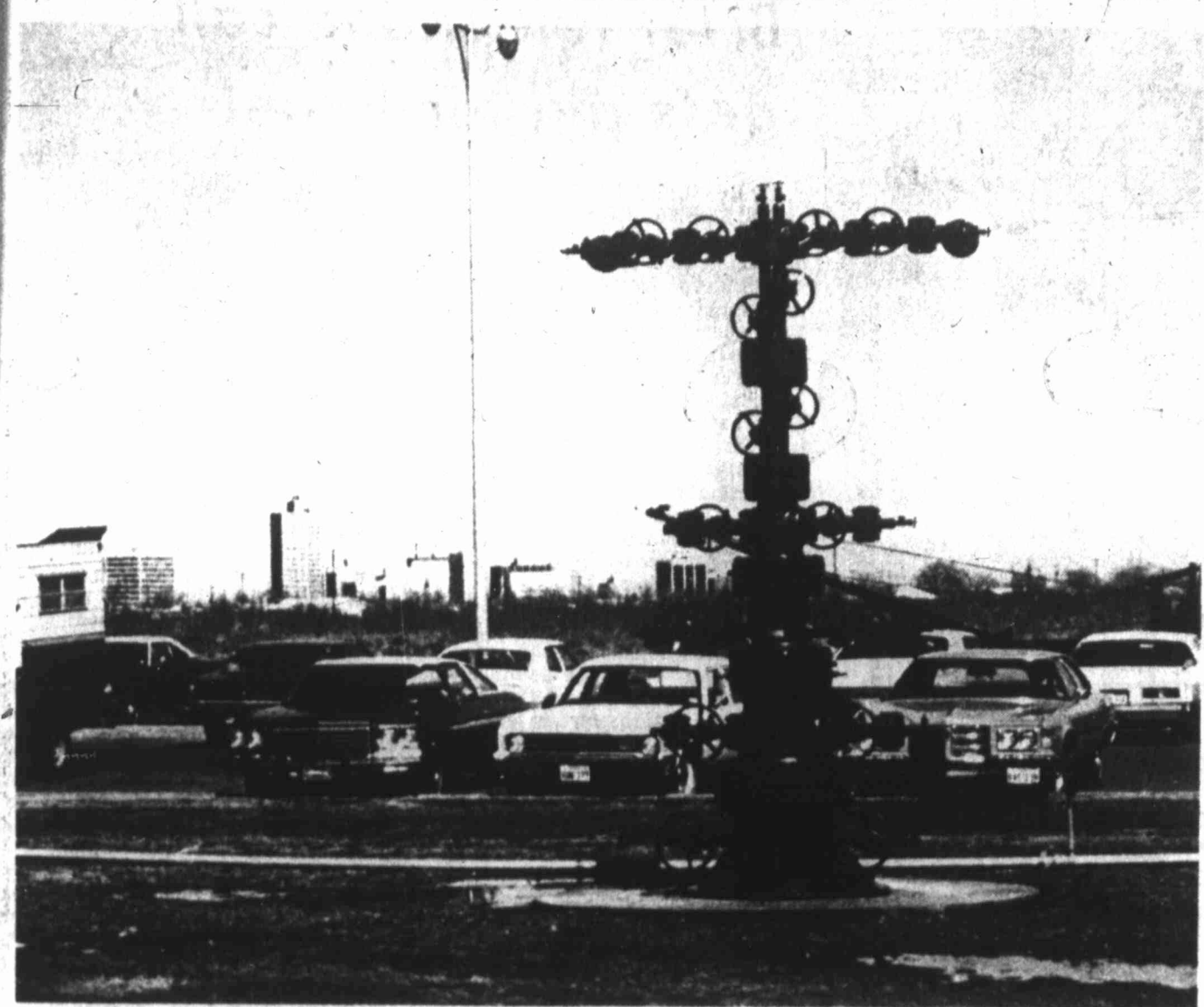
MIDLAND SKYSCRAPERS AND a parking lot full of cars form the background for this picture of one of the Permian Basin Petroleum Museum, Library and Hall of Fame's outdoor exhibits. The array of valves form a "Christmas tree" that controls the flow of oil from a producing well.
