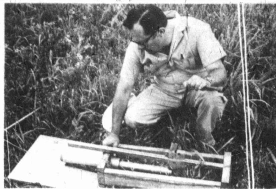
Geologist Bud Johnson watches a sediment core sample extruding from a new tool he devised and tested.
