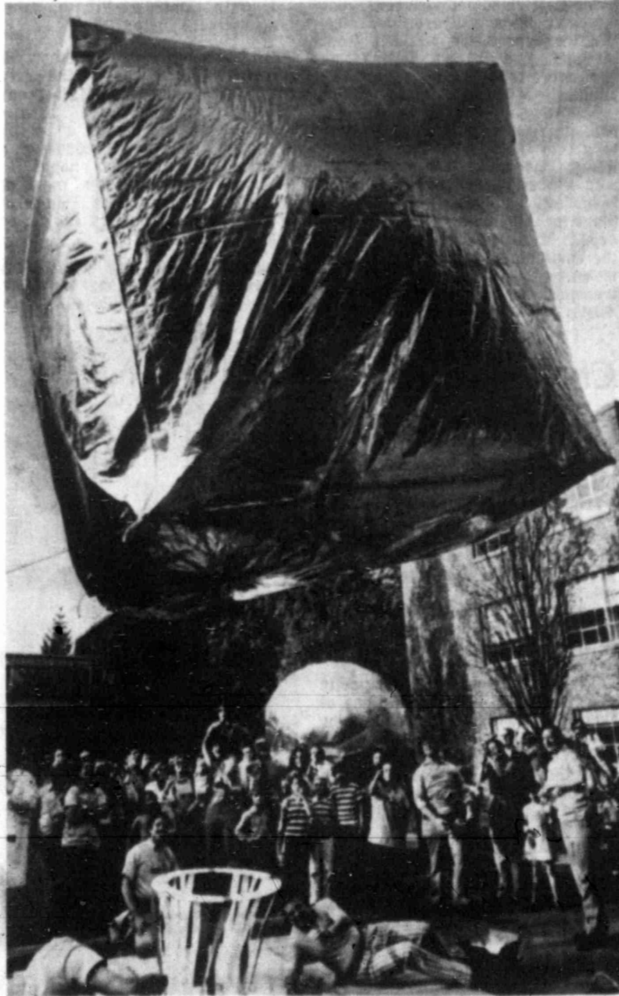
A 729-CUBIC FOOT SQUARE BALLOON made of lead foil and filled with helium gas starts to take off at the Arthur D. Little Inc. research company in Cambridge, Mass. The balloon went up only a few feet before being ripped apart in the breeze. Scientists at Little were attempting to disprove the cliché about lead balloons. (AP Laserphoto)
