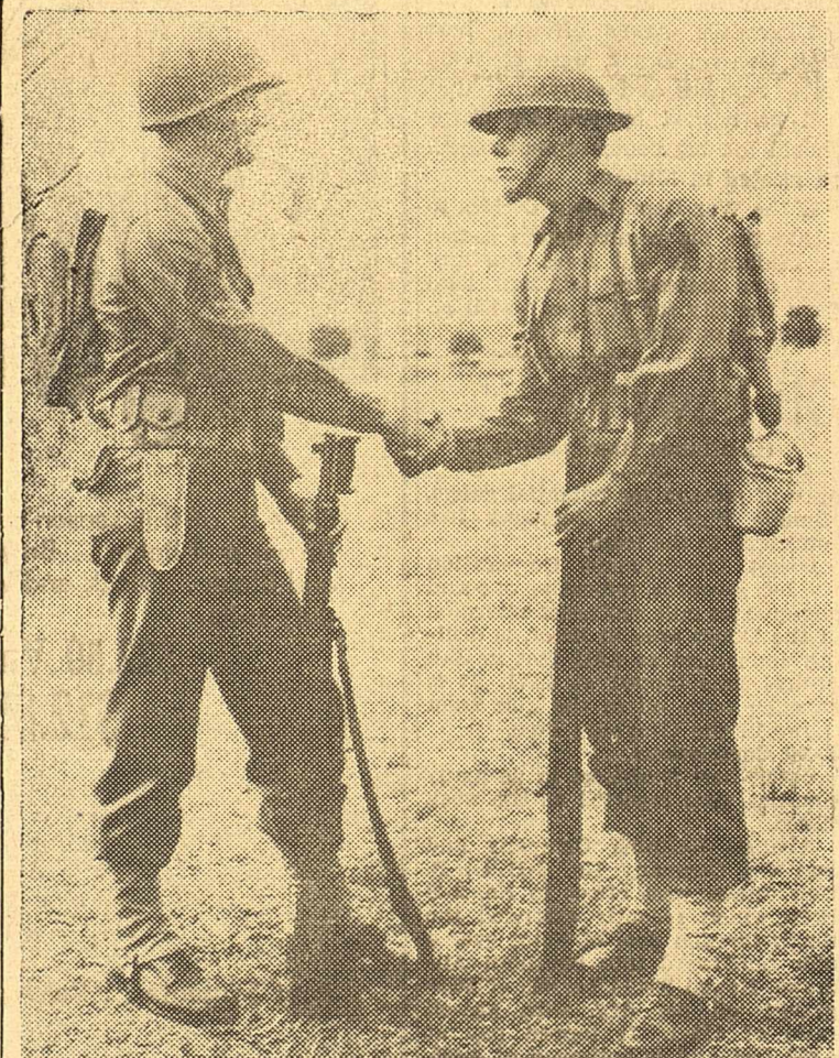
The infantry at Fort Benning, Ga., is testing a proposed new type helmet (worn by soldier at left) which has a fibrous lining designed for use as a field hat. If adopted, the dual purpose helmet will replace the present style (worn by soldier at right). The fibrous lining then may replace the present overseas cap.
