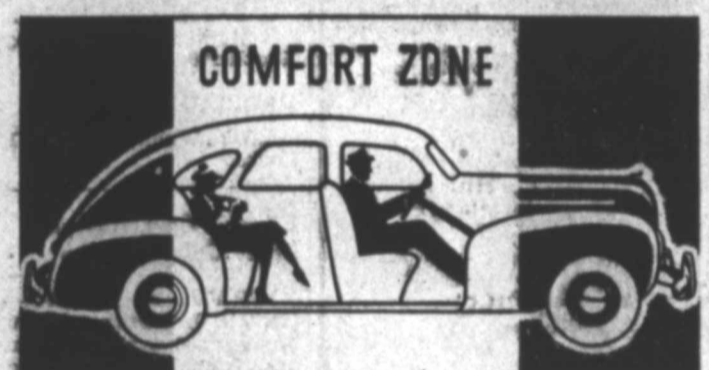
NEW FULL-FLOATING RIDE! Wheelbase is longer, wheels are moved backward, seats forward so that now all passengers ride in the buoyant "Comfort Zone" between the axles!
