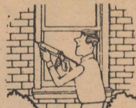
Caulk around doors and windows
