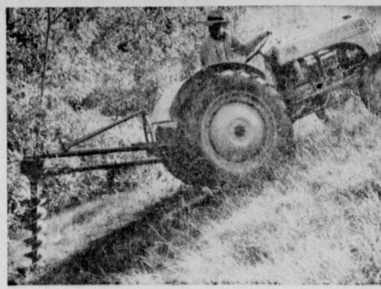
600 HOLES A DAY are now possible with the hydraulically operated digger using power from the tractor's power take-off. Even on hills, as farmer Walt Kemppainen shows above, holes
