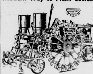
HE McCormick-Deering Farmall 12 Tractor and F-67 1 Planter mounted on it has made a big hit with cotton growers. The F-67 is a 2-row, direct-connected, power-driven planter, easy to mount or remove from the tractor. Each planting unit follows the ground independently of the other, assuring uniform planting depth regardless of variation in the height of the beds.
