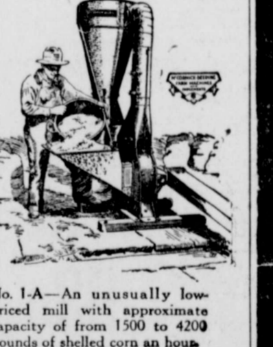
No. 1-A—An unusually low-priced mill with approximate capacity of from 1500 to 4200 pounds of shelled corn an hour.
