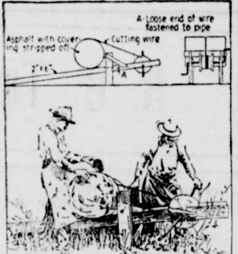
Cutting Asphalt Taken From Barrel With a Wire Drawn Through It With a Windlass.
