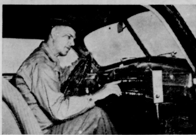
METER MAN . . . Button-filled machine shown in this 1947 photo is not a car radio, but a crop meter. The device, connected to an automobile speedometer, measured the frontage of each crop. Use of aerial photography in crop reporting made it obsolete. U.S. Department of Agriculture has presented a crop meter to the Smithsonian Institution.
