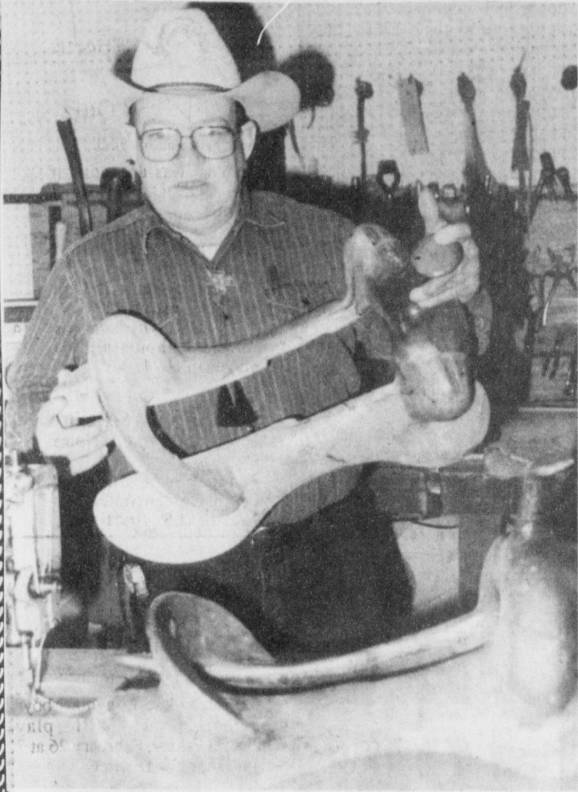
Wooden trees, the top tree is covered with epoxy glass and covered with rawhide.
