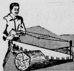
If you want to use a two-man saw alone, run two wires between the handles and put a notched stick between them. This will stiffen the saw and the handles will not wobble from side to side.
