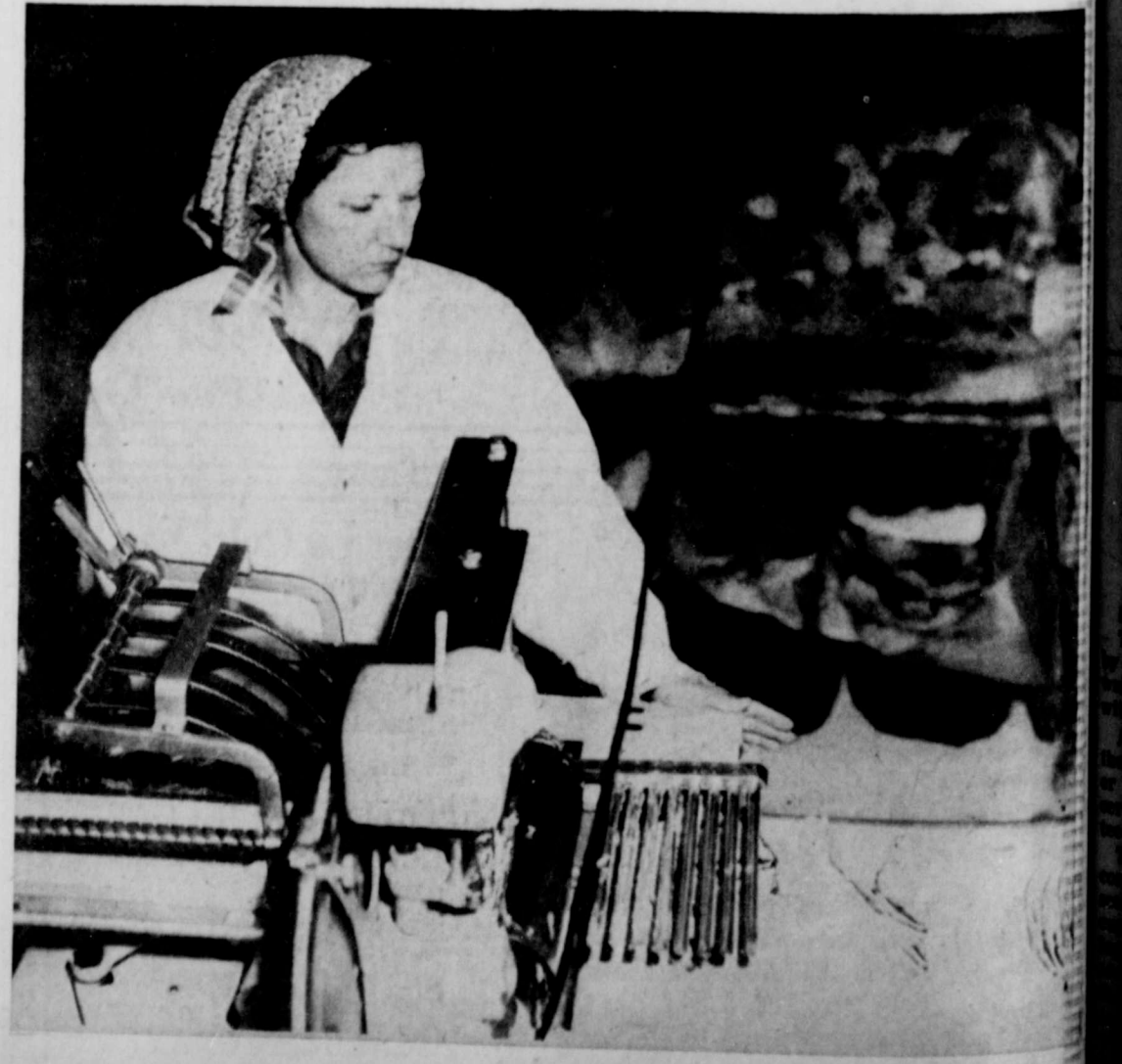
MRS. PAUL RIEGER operates bacon and lunch loaf slicing machine. This is an example of the clean, modern equipment used in Payne packing plant. The machine slices, stocks, and conveys to wrapper and sealer at other end. This bacon, with the long lean strip, is hickory smoked and aged before being sliced, wrapped and shipped.
