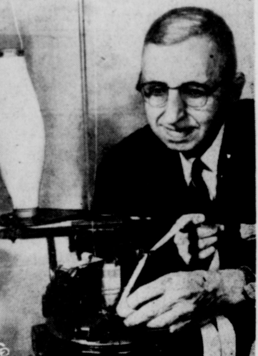
PROFESSOR W. E. SCHINN (right), of North Carolina State College, Raleigh, N. C., works at a machine, used for knitting neckties, which he modified to produce orlon tubing as a substitute for the heart's main artery. Knitted to the proper shape (left), the tubing has been used successfully to replace the aorta in dogs and may soon be used on humans. The orlon remains permanently. (International)
